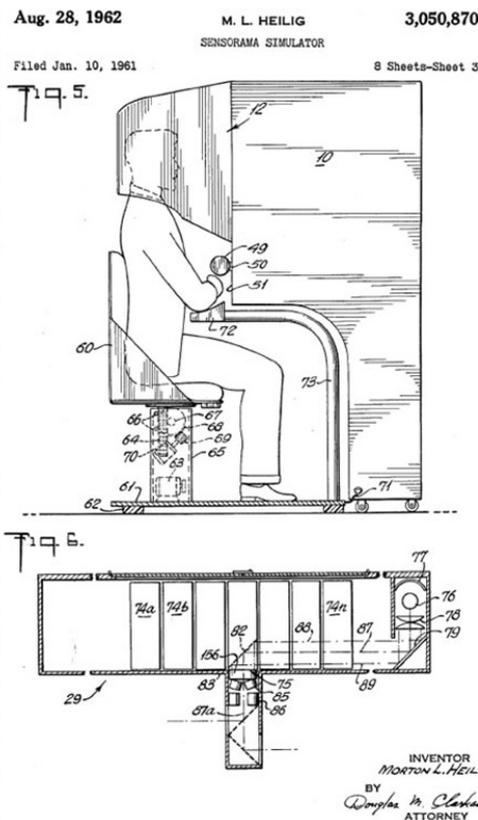
Fig. 1. Sensorama visor system schematics; source: <https://vr-expert.nl/wp-content/uploads/2016/05/sensorama.jpeg>
